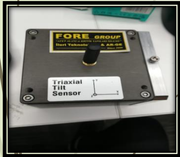
Optical Displacement Sensor + Three-Axis Tilt + Internal Temperature Sensor
